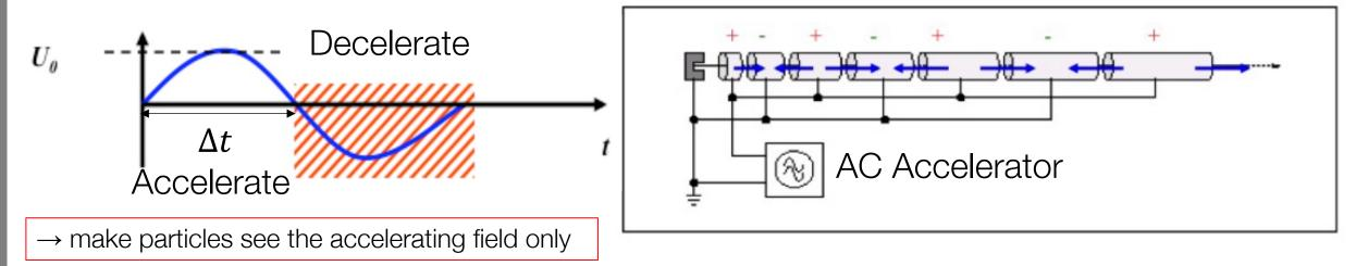
In principle, this device can produce a multiple of the acceleration voltage, if the particles are shielded from the decelerating field (negative half-wave of the AC voltage).
