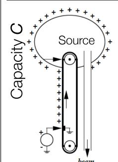
Van de Graaff designed a DC accelerator that used a mechanical transport system to carry charges, sprayed on a belt or chain, to a high-voltage terminal.
