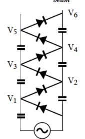
Cockcroft and Walton: acceleration mechanism based on a rectifier circuit, diodes and capacitors.
