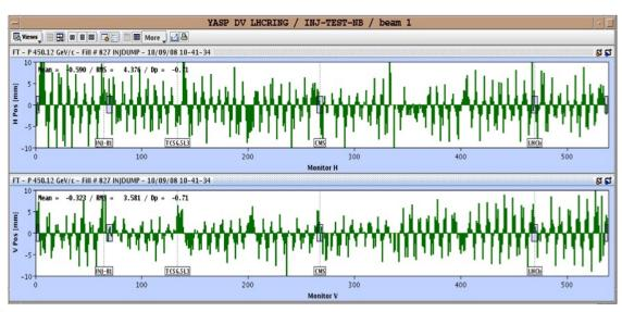
The figure on the left shows the transverse oscillations in the transverse plane of LHC as measured by the monitoring equipment in 1 turn. One important parameter is the the number of oscillations in the horizontal and in the vertical plane
