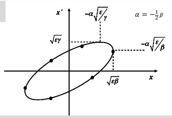
This means that emittance cannot be changed once the optics of the machine is defined: it is a property of the beam.
