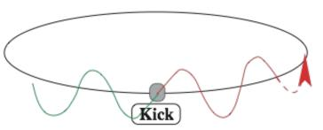
Misalignments, dipole field errors, in one point of the orbit
