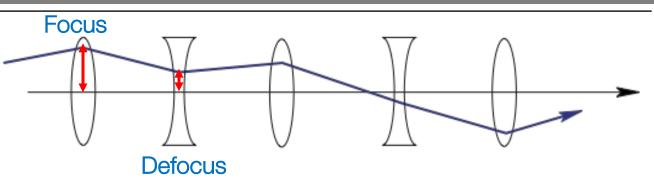
Alternating focusing and defocusing quadrupoles leads to an overall focusing:
