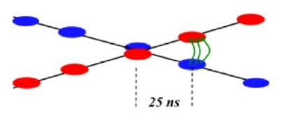
case of a proton—proton collider, this strong field acts like a defocusing lens, and has a strong impact on the tune of the bunches.
