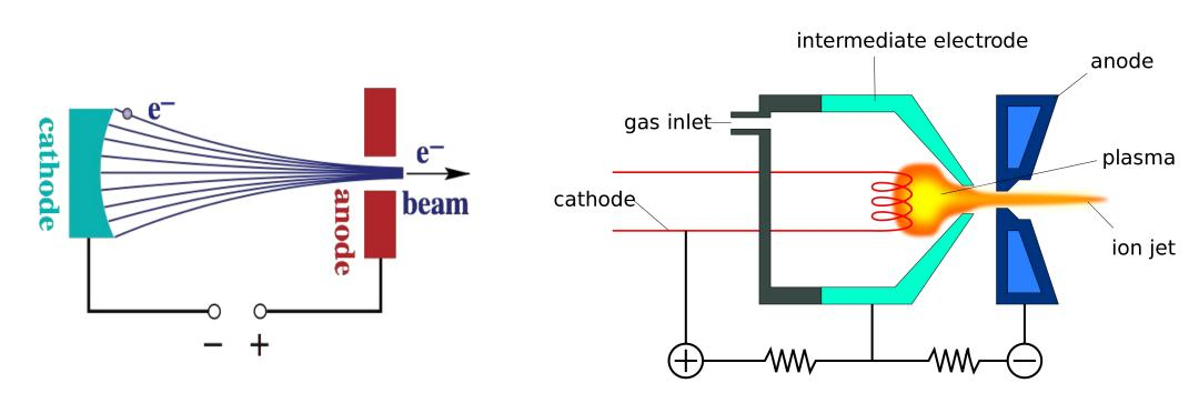
Electron source is based on the thermoionic effect of a filament heated to high temperature. Electrons emitted by the filament are accelerated by an electric field and collimated through a small window.
