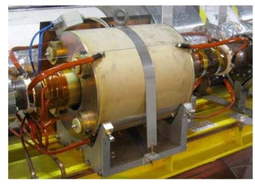
DCCT Beam Current Transformer
