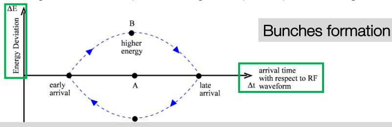
Thus all the particles in the accelerator rotate around the synchronous particle on the longitudinal phase space plot. → instead of being spread uniformly around the circumference of the accelerator
