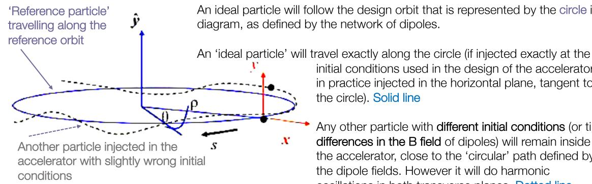
An ideal particle will follow the design orbit that is represented by the circle in the diagram, as defined by the network of dipoles.
